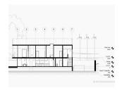
19. Section - A section is an important architectural drawing that allows us to cut through a building and see what it looks like inside.
