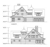
6. Elevation - It is a horizontal orthographic projection of a building that represents one façade of a building.
